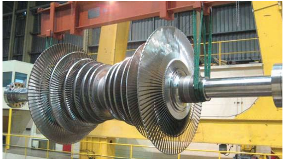
Each unit has four turbines that spin in tandem. Steam first hits a 5-foot diameter high pressure turbine, flows to the 6-foot diameter intermediate turbines and then into two successive low pressure turbines 12-feet in diameter. This photo is a low pressure turbine.
