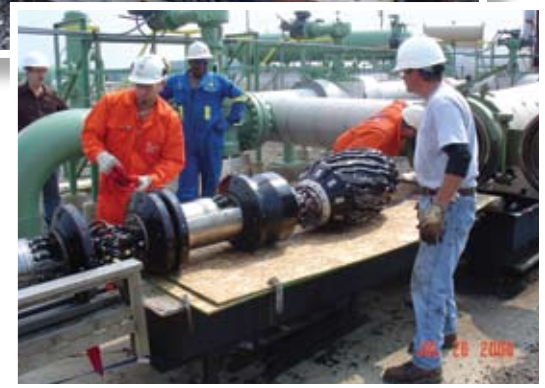
Mark Overholt (right), pipeline attendant for PPL Interstate Energy, checks as a monitoring device known as a "pig," used to check the pipeline for cracks, is removed from the pipeline at the Martins Creek terminal.
