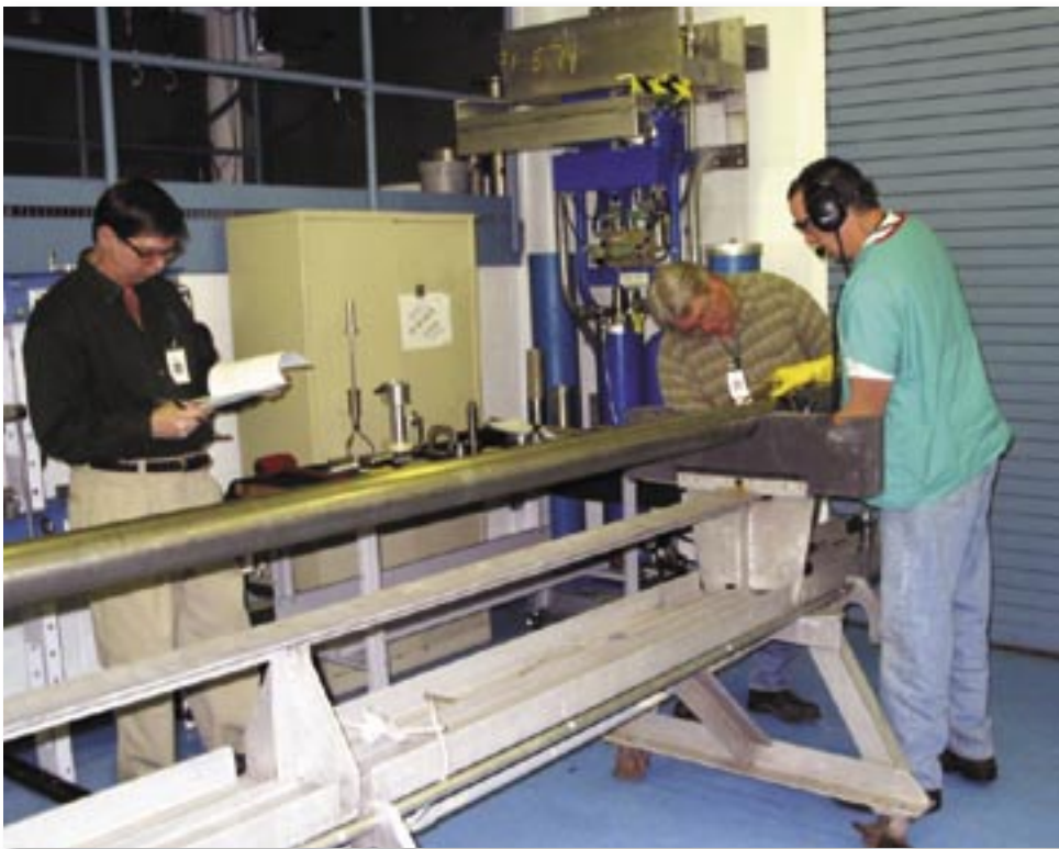
Mechanics rebuild control rod drives every year as part of their annual training. The control rod drives push control rods into the reactor to shut it down.
